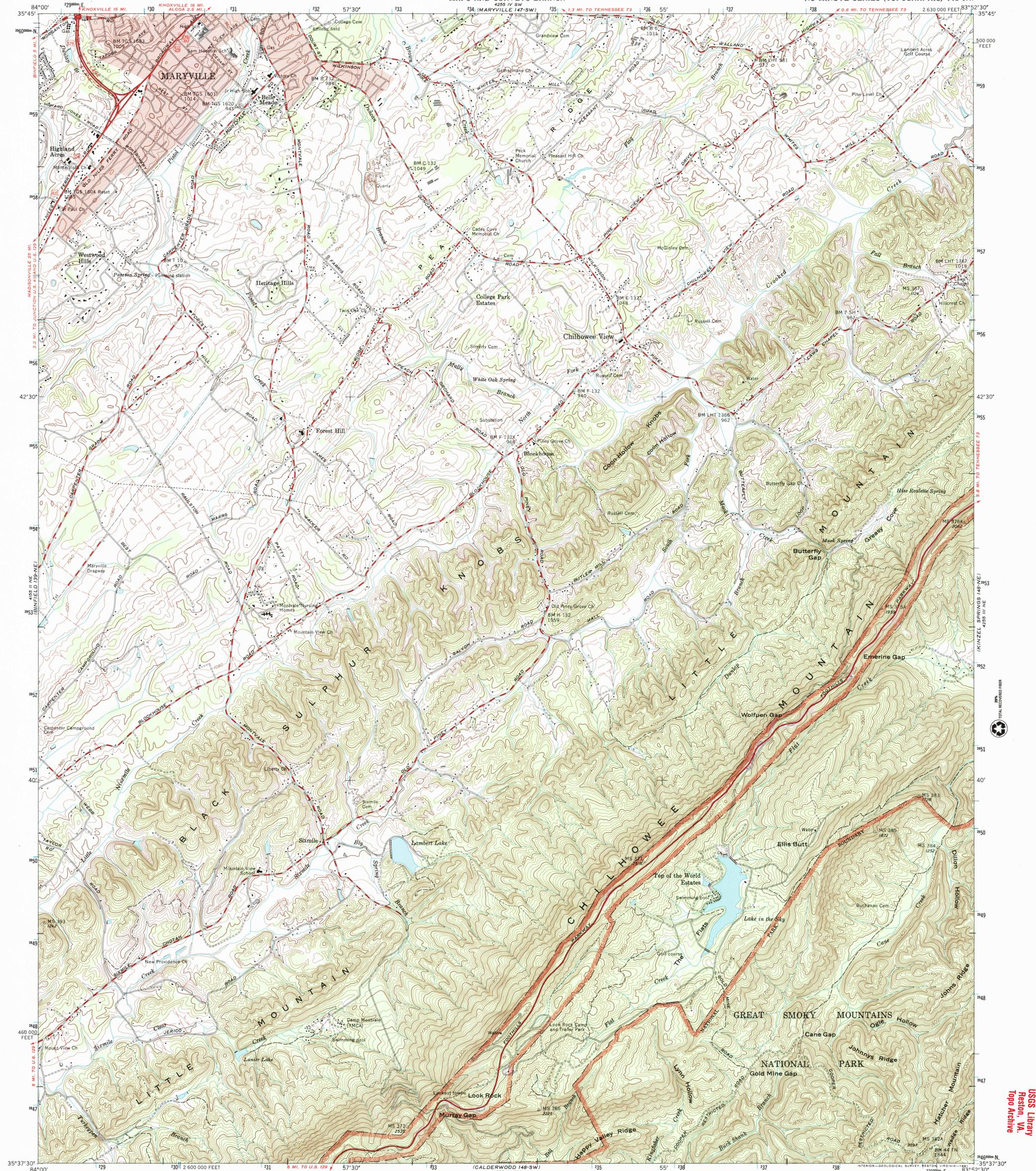
Map published by Tennessee Valley Authority... Control by USGS, USGS, and TVA... Revised by TVA in 1966 by photogrammetric methods... Polyconic projection, 10,000-foot grid ticks based on Tennessee rectangular coordinate system...
